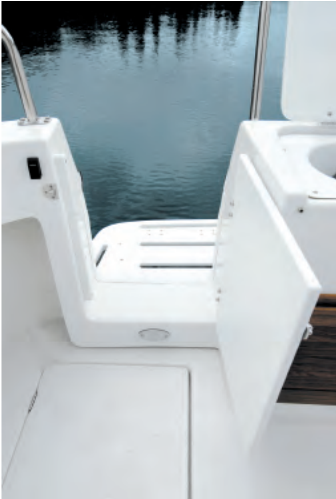
Left: A transom gate offers good access to the swim platform. A cabinet is to the right. The hatch opens to a storage space. Right: Reminiscent of old workboat styling, the blue eyebrows are decorative and deflect rain from the window.
