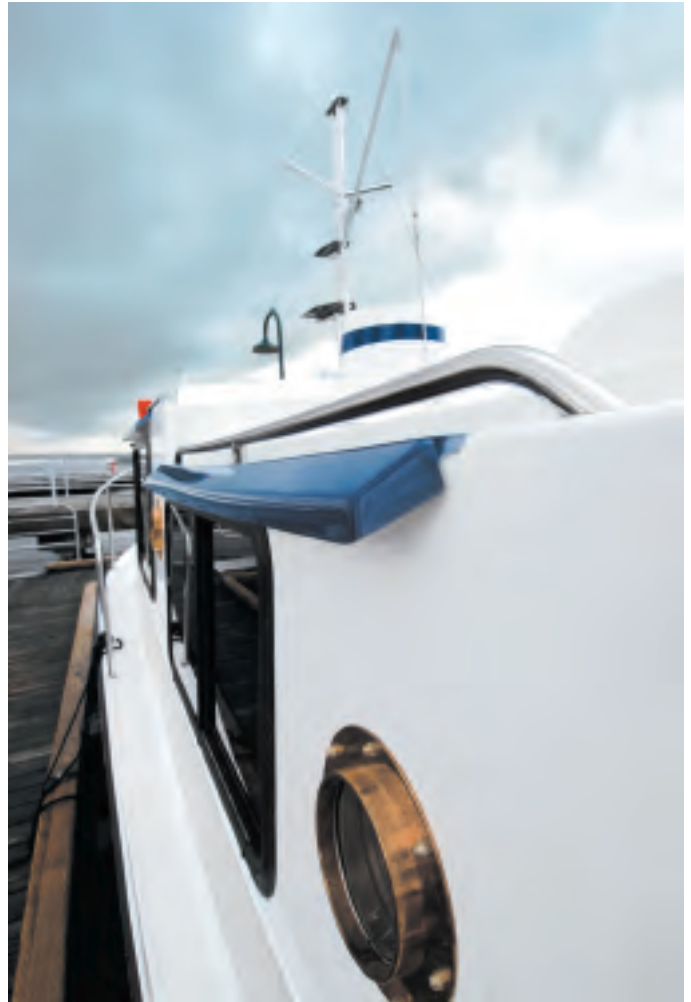
Left: A transom gate offers good access to the swim platform. A cabinet is to the right. The hatch opens to a storage space. Right: Reminiscent of old workboat styling, the blue eyebrows are decorative and deflect rain from the window.
