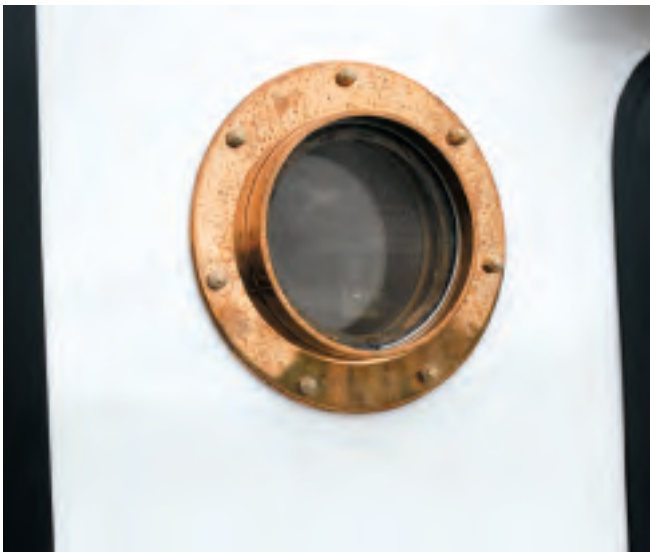
Top: A pantry shelf in the galley with an opening portlight. Above: Portlights are a strong design feature on the R25. Seen from the outside and the inside, they are salty and practical, and they open for improved ventilation.
