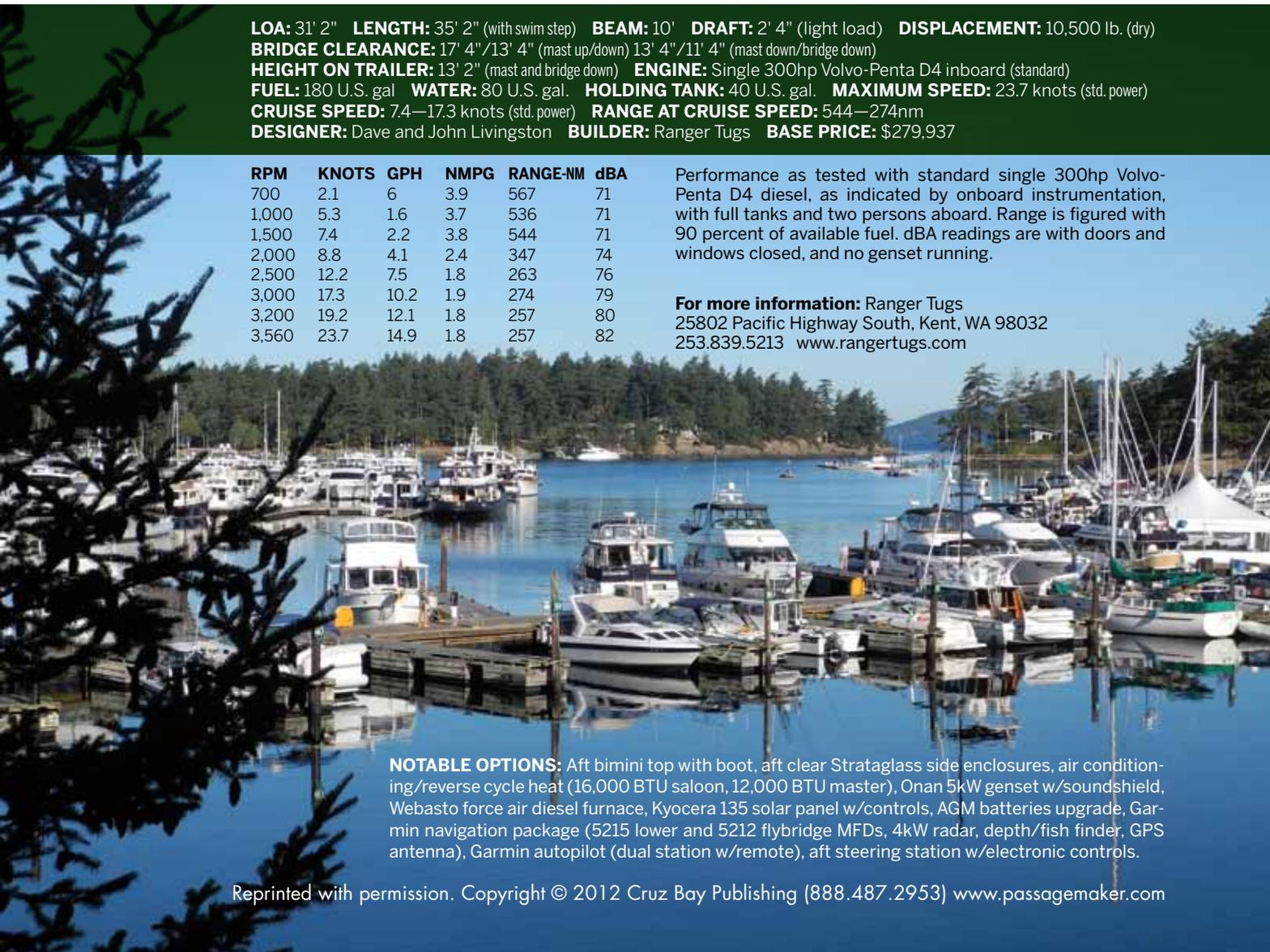
**NOTABLE OPTIONS:** Aft bimini top with boot, aft clear Strataglass side enclosures, air conditioning/reverse cycle heat (16,000 BTU saloon, 12,000 BTU master), Onan 5kW genset w/soundshield, Webasto force air diesel furnace, Kyocera 135 solar panel w/controls, AGM batteries upgrade, Garmin navigation package (5215 lower and 5212 flybridge MFDs, 4kW radar, depth/fish finder, GPS antenna), Garmin autopilot (dual station w/remote), aft steering station w/electronic controls.
