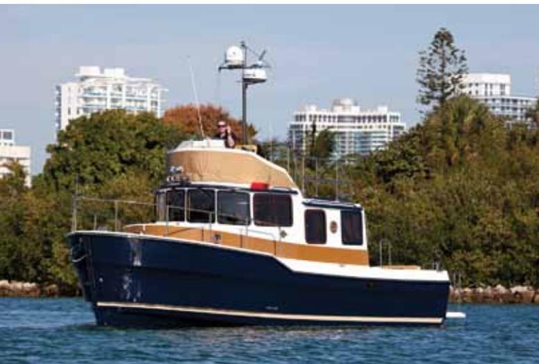
*The flybridge is lightweight owing to its use of wraparound canvas instead of solid fiberglass. Thus, the bridge can be folded forward for passing under low bridges.*
