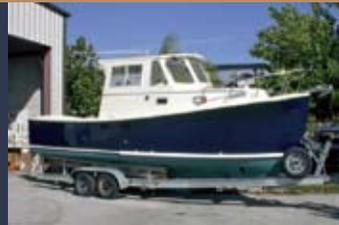
**LOA:** 24 feet, 10 inches **BEAM:** 8 feet, 6 inches **DRAFT:** 2 feet, 6 inches **WEIGHT:** 5,100 pounds **HULL TYPE:** semidisplacement **TANKAGE:** 60 gallons fuel, 20 gallons water **POWER:** single diesel to 180 hp **SPEED:** 20-22 mph **PRICE:** \$96,337 **CONTACT:** Atlas Boat Works, Cape Coral, Fla. Phone: (239) 574-2628. [www.acadia25.com](http://www.acadia25.com)
