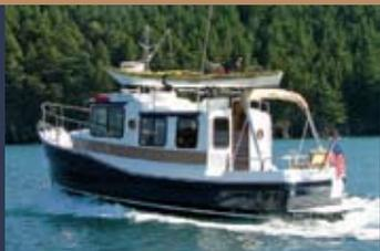
**LOA:** 24 feet, 7 inches **BEAM:** 8 feet, 6 inches **DRAFT:** 2 feet, 2 inches **WEIGHT:** 5,700 pounds **HULL TYPE:** semidisplacement **TANKAGE:** 75 gallons fuel, 30 gallons water **POWER:** diesel to 150 hp **SPEED:** 16-17 mph **PRICE:** \$119,940 **CONTACT:** Ranger Tugs, Kent, Wash. Phone: (253) 839-5213. [www.rangertugs.com](http://www.rangertugs.com)
