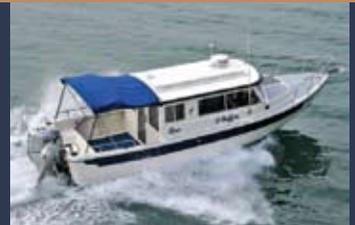
**LOA:** 25 feet, 5 inches **BEAM:** 8 feet, 6 inches **DRAFT:** 10 inches **WEIGHT:** 3,600 pounds **HULL TYPE:** semidisplacement **TANKAGE:** 100 gallons fuel, 23 gallons water **POWER:** single 150- or twin 90-hp outboards **SPEED:** 30 mph (top) **PRICE:** \$59,085 (without power) **CONTACT:** C-Dory Marine Group, Auburn, Wash. Phone: (253) 839-0222. [www.c-dory.com](http://www.c-dory.com)
