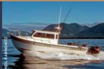
**LOA:** 26 feet **BEAM:** 8 feet, 6 inches **DRAFT:** 1 foot, 6 inches **WEIGHT:** 6,500 pounds **HULL TYPE:** semidisplacement **TANKAGE:** 150 gallons fuel, 30 gallons water **POWER:** single gas or diesel inboard, single or twin outboards **SPEED:** 30 mph (top) **PRICE:** \$150,656 (with 250-hp diesel) **CONTACT:** Osprey Boats, Bellingham, Wash. Phone: (360) 738-4671. [www.ospreyboats.com](http://www.ospreyboats.com)
