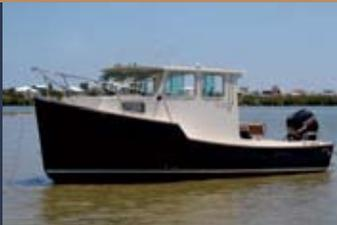
**LOA:** 21 feet **BEAM:** 8 feet, 6 inches **DRAFT:** 9 inches **WEIGHT:** 2,350 pounds **HULL TYPE:** semidisplacement **TANKAGE:** portable fuel and water tanks **POWER:** single outboard to 70 hp **SPEED:** 20 mph cruise **PRICE:** \$32,900 **CONTACT:** Retro Marine, Salem, Mass. Phone: (978) 578-1606. [www.retromarine.com](http://www.retromarine.com)
