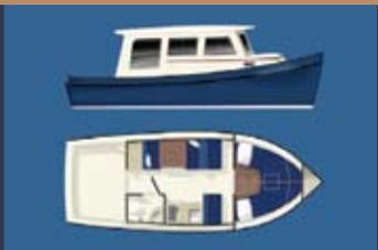
**LOA:** 25 feet **BEAM:** 8 feet, 6 inches **DRAFT:** 1 foot, 4 inches **WEIGHT:** 4,700 pounds **HULL TYPE:** semidisplacement **TANKAGE:** 80 gallons fuel, 37 gallons water **POWER:** single outboard to 175 hp, single diesel to 190 hp **SPEED:** 18-20 mph **PRICE:** \$99,000 (with 150-hp outboard) **CONTACT:** Seaway Boats, Oxford, Maine. Phone: (207) 539-8116. [www.seawayboats.com](http://www.seawayboats.com)
