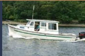
**LOA:** 25 feet **BEAM:** 8 feet, 6 inches **DRAFT:** 1 foot, 6 inches **WEIGHT:** 5,400 pounds **HULL TYPE:** semidisplacement **TANKAGE:** 120 gallons fuel, 42 gallons water **POWER:** single or twin outboards to 300 hp, single gas or diesel sterndrive **SPEED:** 15-20 mph **PRICE:** \$87,400 (without power) **CONTACT:** Rosborough Boats, Halifax, Nova Scotia. Phone: (902) 450-3262. [www.rosboroughboats.com](http://www.rosboroughboats.com)
